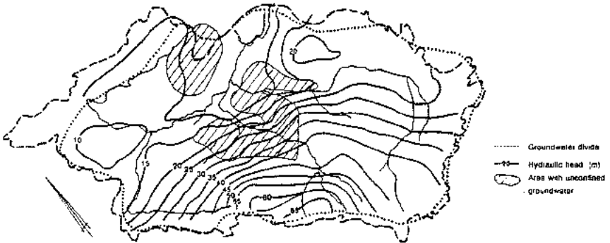
Fig.4 The hydraulic head in the regional aquifer and areas with unconfined groundwater.
